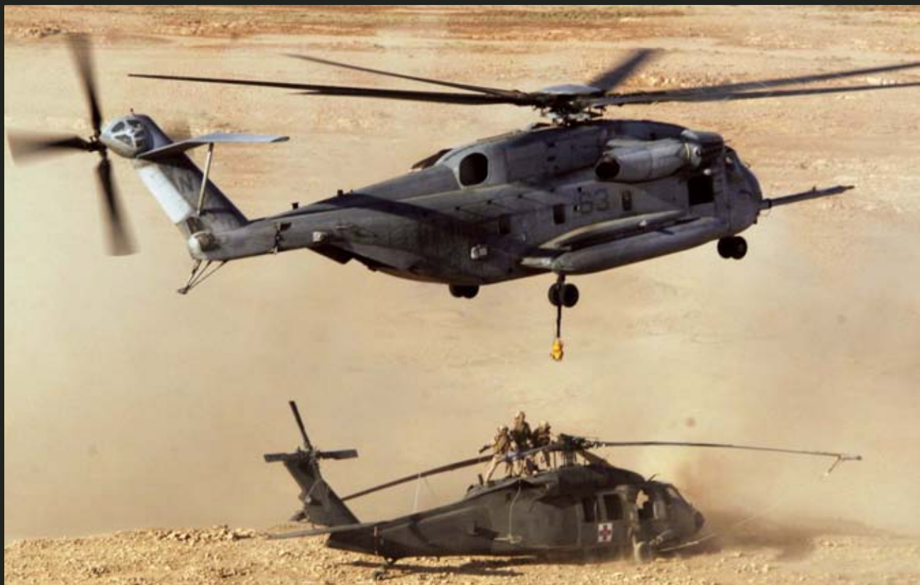
BLACKHAWK DOWN? NOT A PROBLEM FOR MARINE SUPER STALLION —Helicopter Support Team leathernecks prepare to hook an Army UH-60 Blackhawk to a CH-53E Super Stallion of Marine Heavy Helicopter Squadron 361 on Sept. 27. The Army chopper was disabled during a routine mission, and Marines gladly provided a helping hand. The HST Marines were from Combat Logistics Company 111, Combat Logistics Battalion 1, First Marine Logistics Group (Forward).
